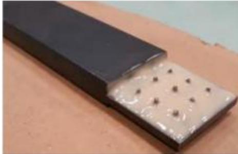
Nota: Ilustración tomada de Design, manufacturing and testing of hybrid adhesive joints with metallic pins to join steel with fiberglass reinforced composite, (Arenas, 2019).
