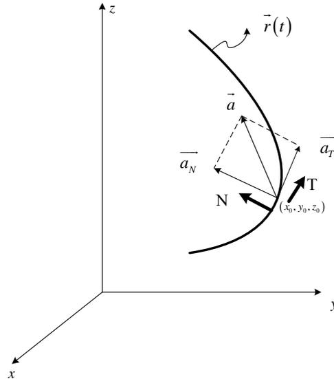
$$\begin{aligned}\vec{a} &= \vec{a}_T + \vec{a}_N \\ &= a_t \mathbf{T} + a_n \mathbf{N}\end{aligned}$$
