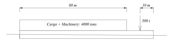
Weight of the hull is 2000 tons, uniformly distributed on the length of the ship; weight of cargo and machinery is 4000 tons, uniformly distributed on the aft part of the ship, as shown in the figure. There is also machinery in the ship's forward end, which can be assumed as a concentrated force of 500 tons.
