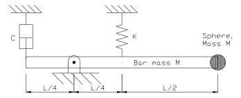
3.- A model to analyze the system to operate valves is depicted in the following figure. The massless actuator ("lifter") moves vertically with harmonic motion, y(t). Determine the amplitude of the resulting motion. (25)
