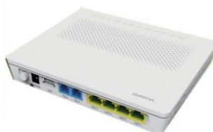
Figura 3.11: Optical Network Terminal (ONT) HG8245 [6]
