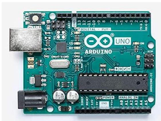
Figura 1.18 Placa Arduino [26]
