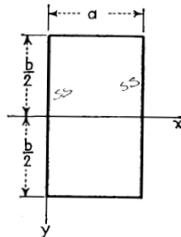
TABLE 35. DEFLECTIONS AND BENDING MOMENTS IN A UNIFORMLY LOADED RECTANGULAR PLATE WITH BUILT-IN EDGES (FIG. 91)  $\nu = 0.3$
