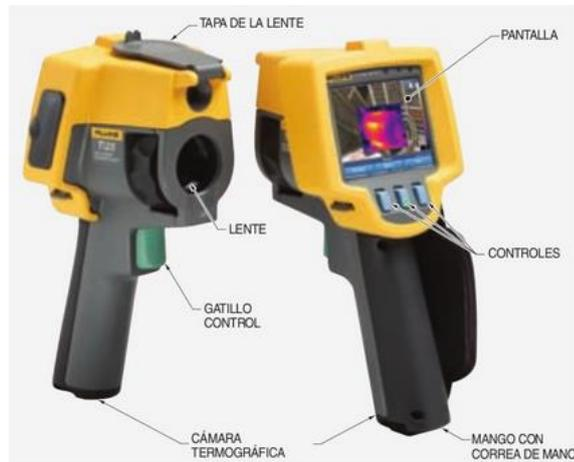
**FIGURA 2.11 CÁMARA TERMOGRÁFICA**
