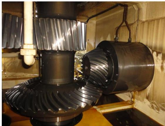
**FIGURA 3.13 INTERIOR DEL REDUCTOR CAJA #2**
