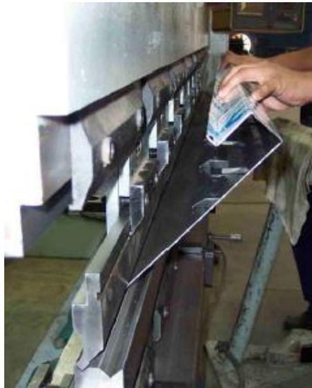
Fig. 2. - Prensado (Press brake operation)
