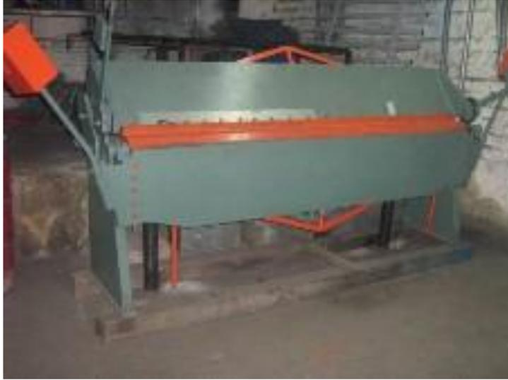
Fig. 3. - Doblado (Bending brake operation)
