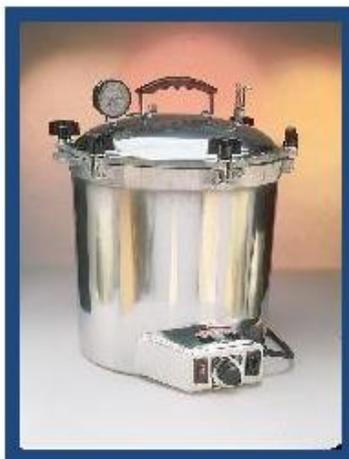
Completely self-contained sterilizers have an immersion heating element, automatic thermostatic control, automatic release valve, and pilot light. Ensure complete, efficient sterilization. Only a small amount of water is needed, and the dry steam, at a temperature of 135°C (275°F), penetrates bandages or instruments, making them sterile in 20 or 30 minutes.
