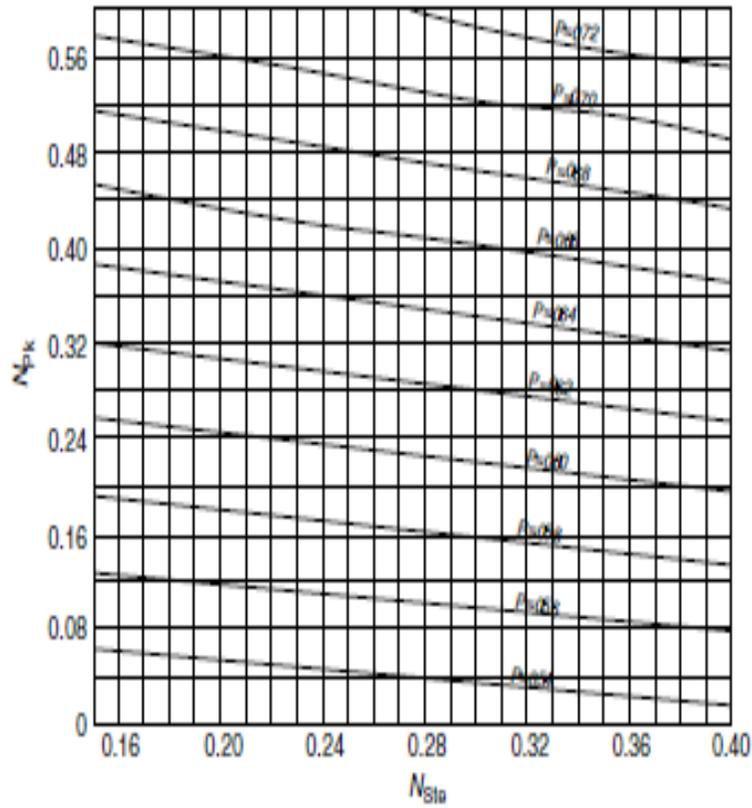
**FIGURE 6.10** Chart showing the Planck number vs. the Stefan number for determination of different values of the empirical modification  $P$ . (From Cleland, A.C. and Earle, R.L. 1982. *Int. J. Refrig.* 5: 134–140. With permission.)
