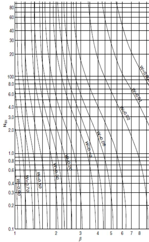
**FIGURE 6.12** Chart showing the Biot number vs. the shape factor for determination of different values of  $W$ .
