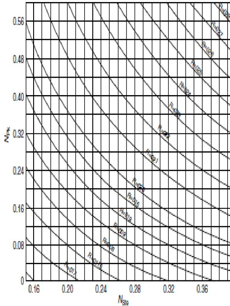
**FIGURE 6.11** Chart showing the Planck's number vs. the Stefan number for determination of different values of the empirical modification  $P$ . (From Cleland, A.C. and Earle, R.L. 1982. *Int. J. Refrig.* 5: 134–140. With permission.)
