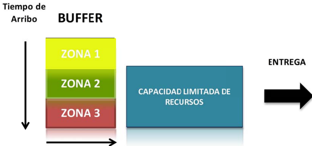
FIGURA 2.6. DBR Amortiguadores de tres Zonas FUENTE: Mark J. Woepel (2003), Manufactured's Guide to Implementing the Theory of Constrains .
