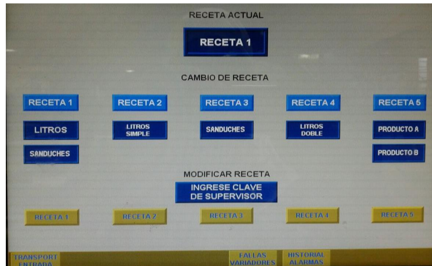
Figura 3.1 Panel View: Barra de Recetas
