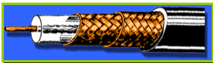
Figura 7.20 Cable Coaxial BELDEN 8281
