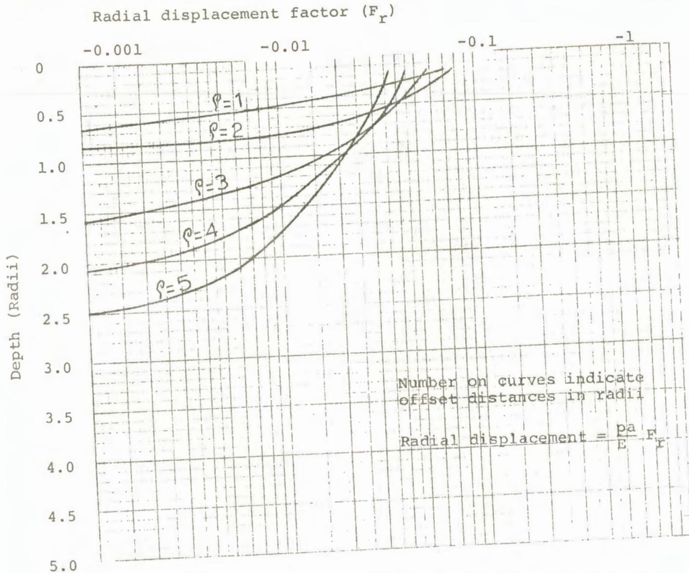
Chart 9. Radial displacement (Poisson's ratio = 0.35)
