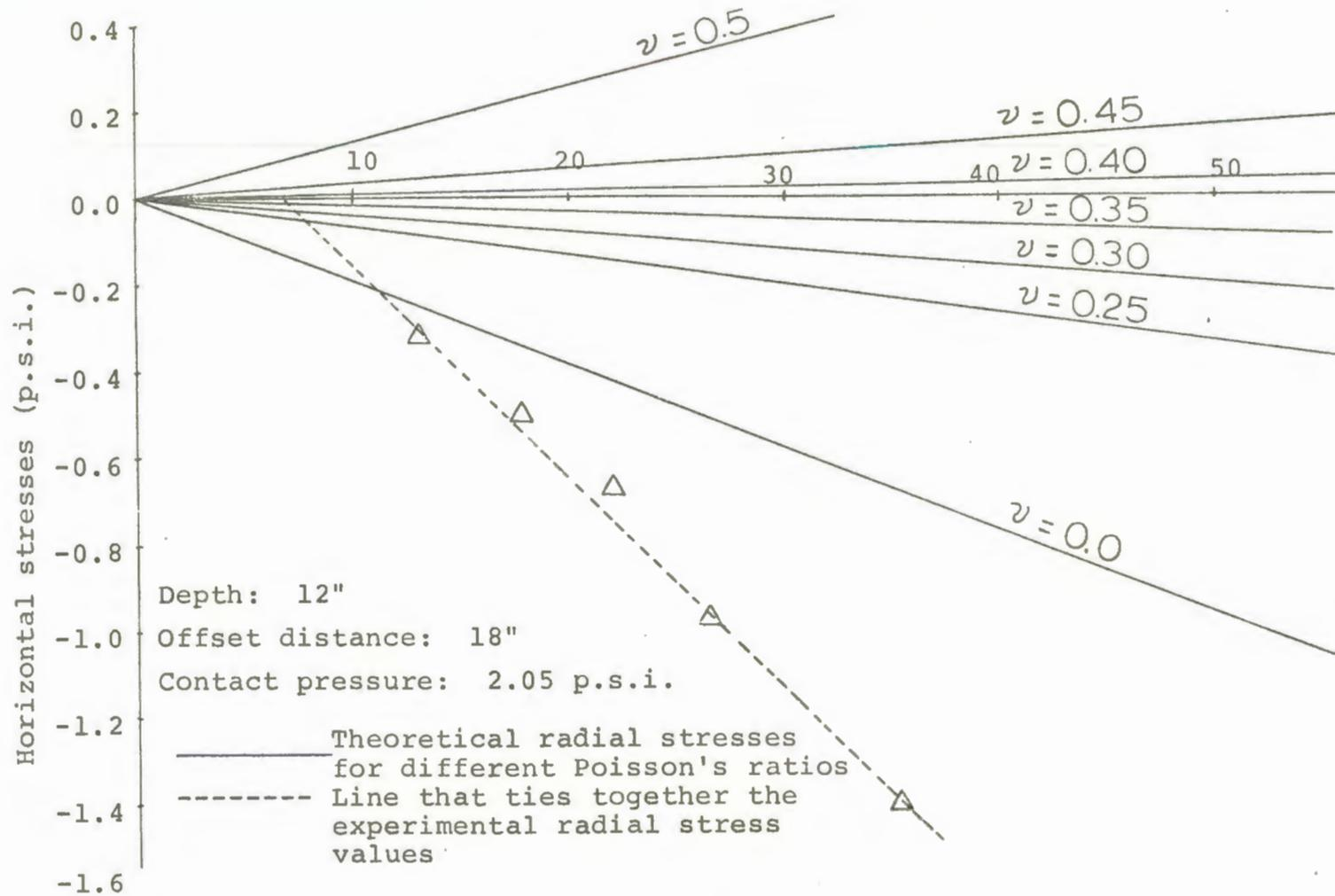
Figure 15. Recorded experimental stresses that correspond to displacements allowed by a material whose Poisson's ratio is 0.3
