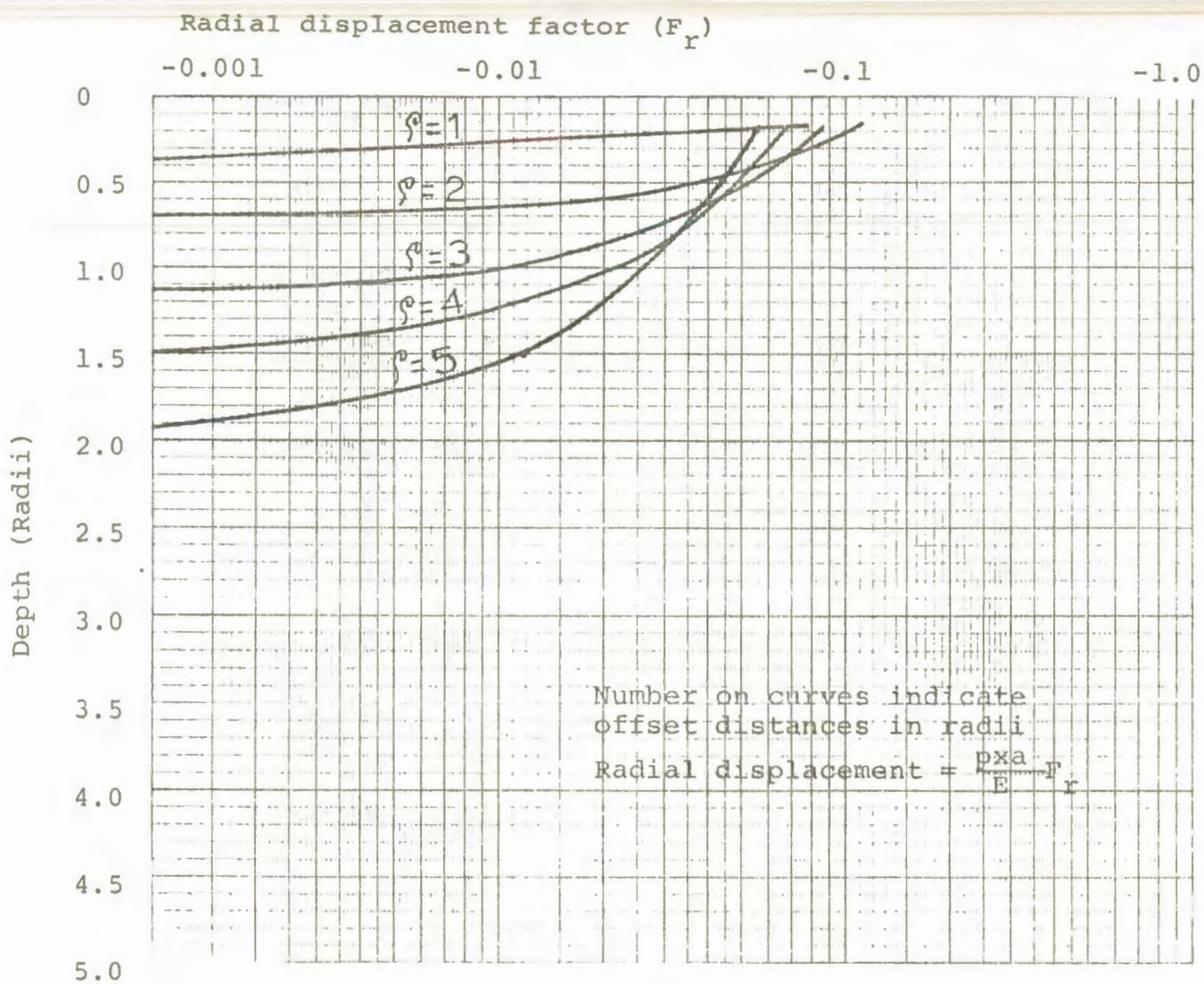
Chart 7. Radial displacement (Poisson's ratio = 0.25)
