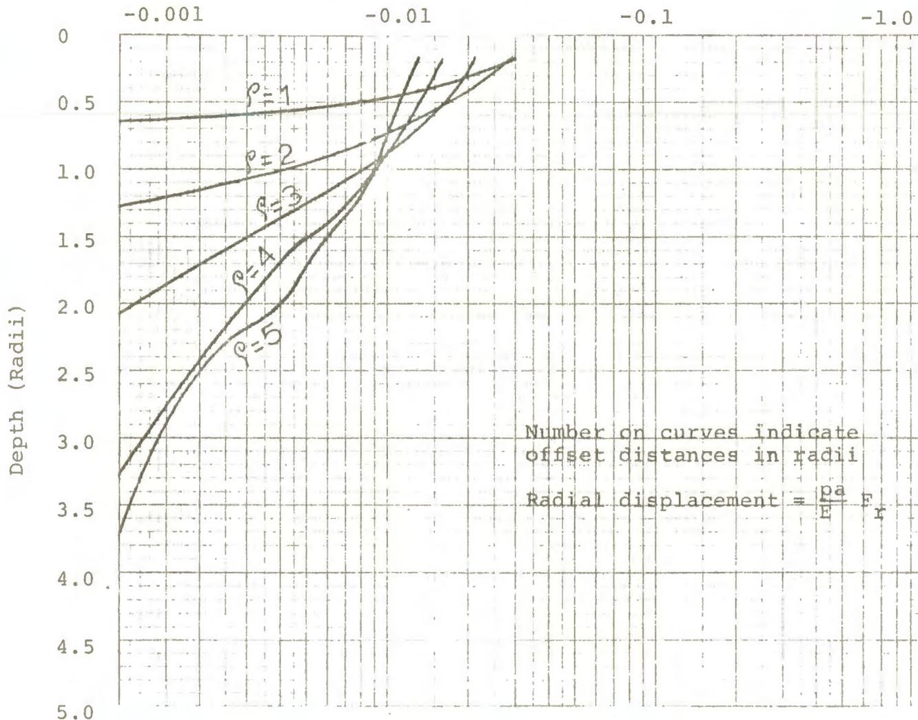
Chart 11. Radial displacement (Poisson's ratio = 0.45)
