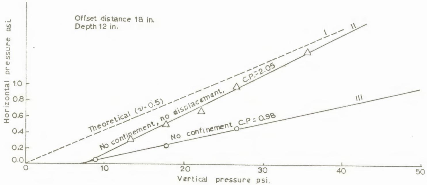
Figure 9. Recorded experimental stresses when no radial displacement was allowed
