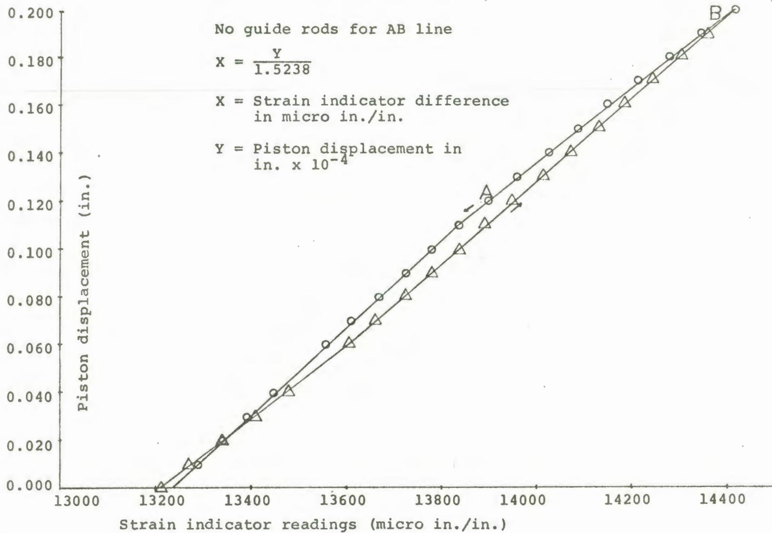
Figure 16. Piston displacement vs. strain indicator readings
