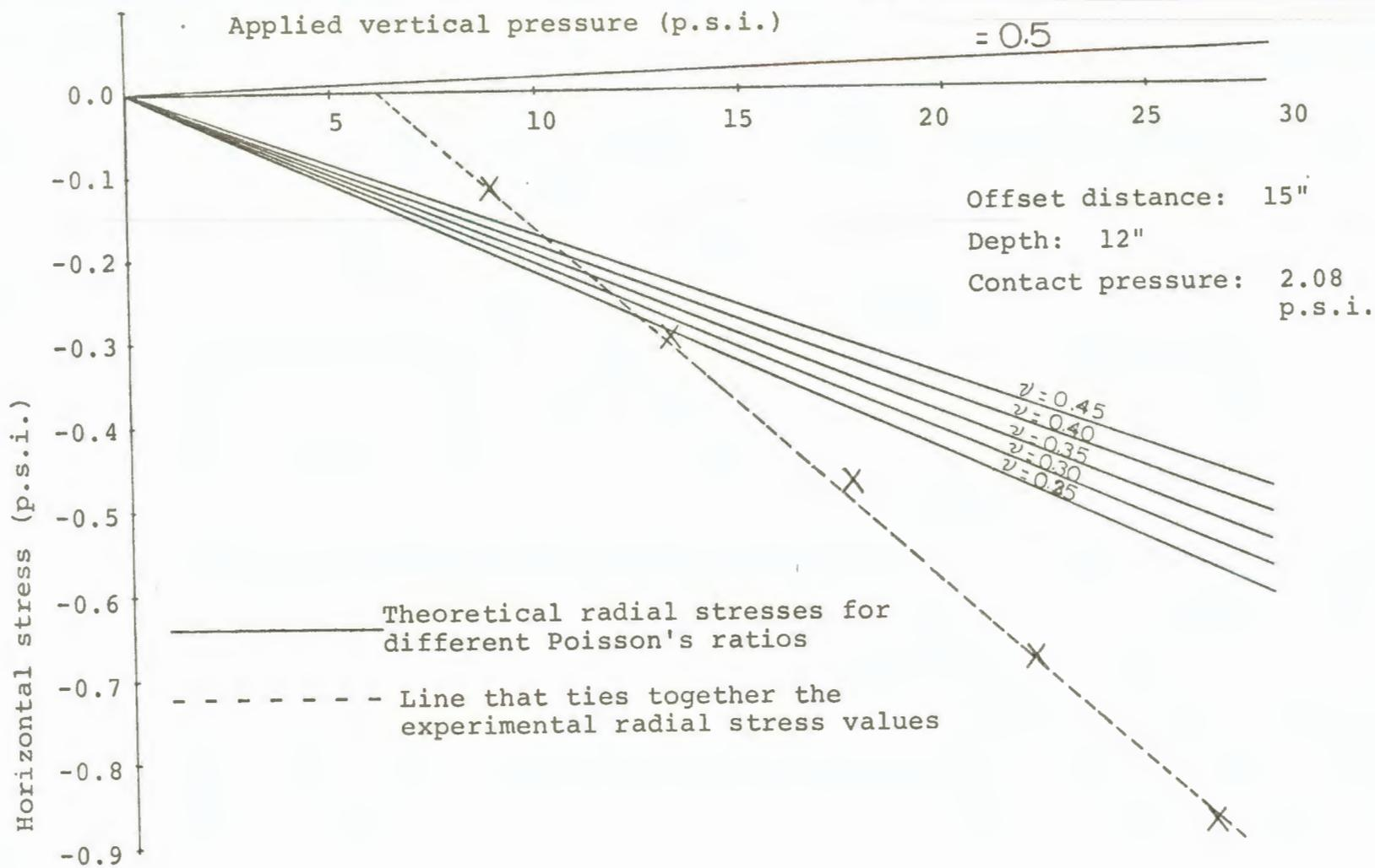
Figure 14. Recorded experimental stresses that correspond to displacements allowed by a material whose Poisson's ratio is 0.3
