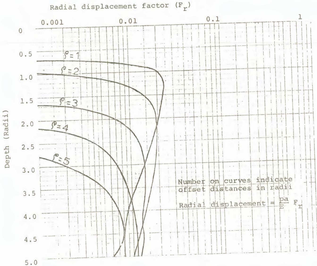
Chart 10. Radial displacement (Poisson's ratio = 0.35)
