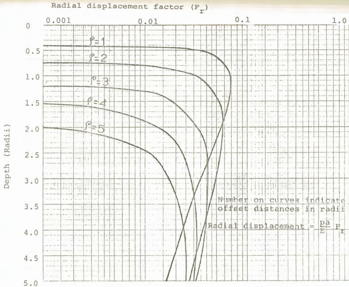
Chart 8. Radial displacement (Poisson's ratio = 0.25)
