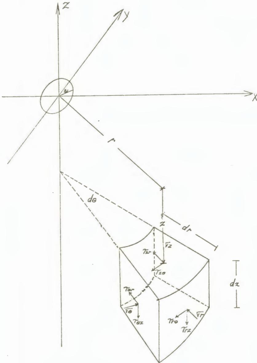
Figure 12. Stresses acting on an infinitesimal element located at depth  $z$  and offset distance  $r$  from the center of the plate
