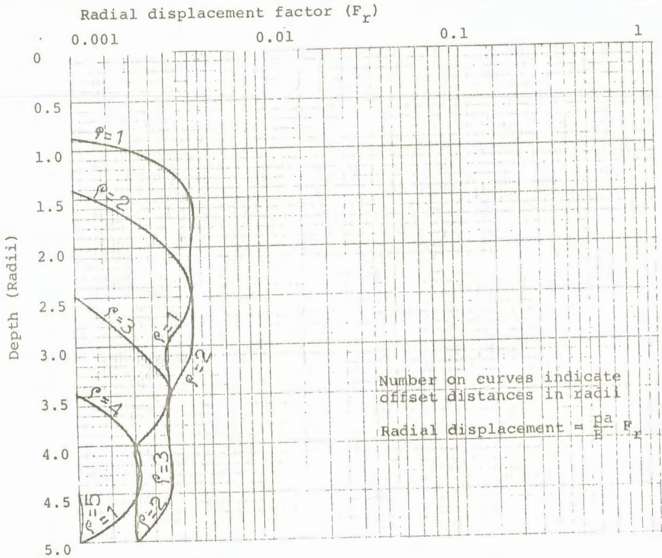
Chart 12. Radial displacement (Poisson's ratio = 0.45)
