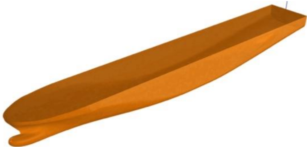
Figure 15: Perspective view of DTC Hull
