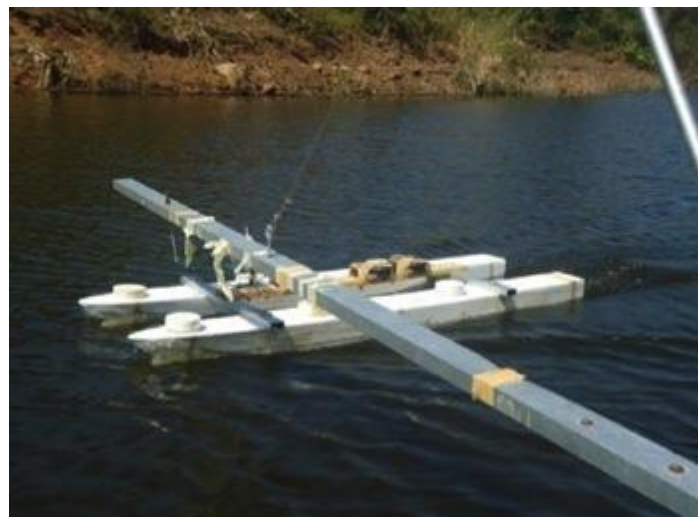
Figure 5: Experimental twin hull test at ESPOL lake in Full Load Condition
