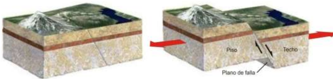
Figure 1.3 Structure of a Normal Fault. (INPRES, 2013).
