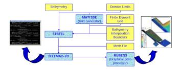
TELEMAC 2D runs in a DOS environment, in function of the Steering file settings (initial, boundary and numerical options). The geometry, boundary and liquid boundary (Water Level) files are defined inside the Steering file to be read by TELEMAC 2D. The model results are processed in RUBENS, the postprocessor, to compare them with observed velocities and calibrate the model.
