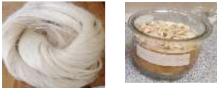
Figure 1 cabuya fiber before and after treatment
