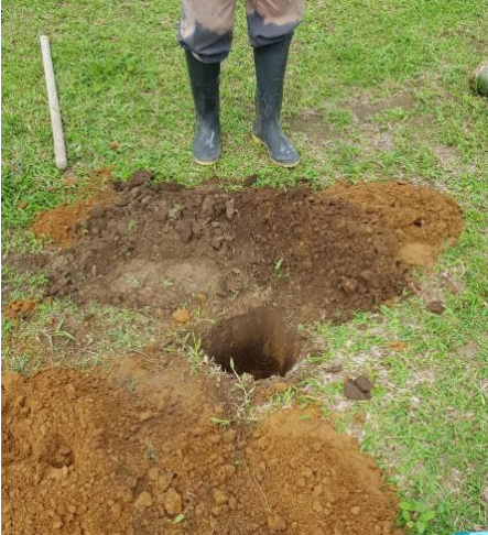
Figura 2.7 Calicata 1. [Pelayo & Ashby, 2020]
