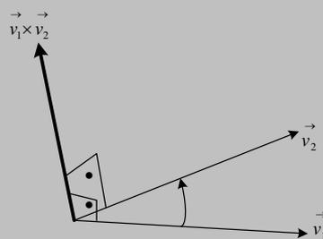
$$3. \vec{v}_1 \times \vec{v}_2 = -\left(\vec{v}_2 \times \vec{v}_1\right)$$
